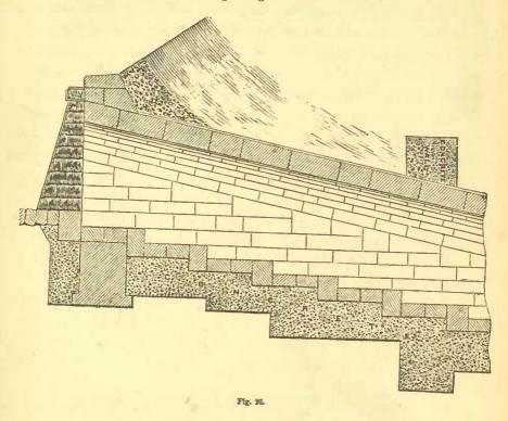
The line of paving was placed considerably lower than the natural bed of the stream; the whole masonry was laid in cement; and the walls at the upper end were built in such a way as to be impervious to water.
